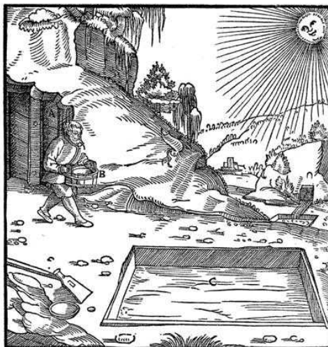
Woodcut from the book de re metallica written by Georgius Agricola (1494 - 1555) illustrating the manual recovery of copper-containing mine effluents which are collected in wooden basins and concentrated in the sun.
