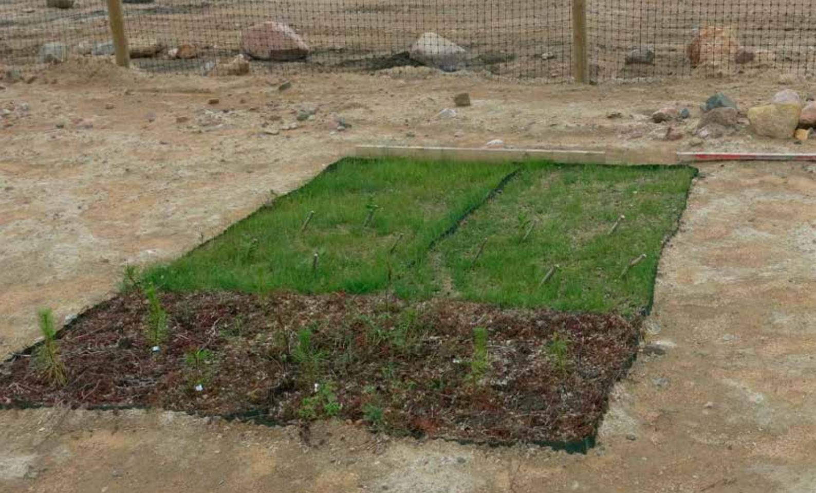
The greening of waste areas is being studied in the Rautuvaara tailings area under natural conditions by using different cover solutions, seed mixtures and plants.
