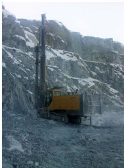
Eti Bakır Murgul copper mine is owned by Cengiz İnsaat using ROC L8 drill rigs at their open-pit copper mine. They are drilling with Atlas Copco Down the hole hammer 165 mm.
